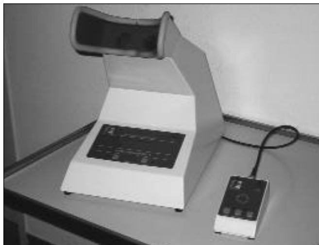
Fig. 1 - Kontrastometer BA4, table mounted look-in device with operator's external control.
